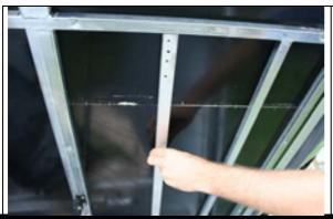
Add 2cm thick steel, aluminium or wood sections where the frame is not sitting on top of the trailer walls to allow your trailer to be sealed later on.
