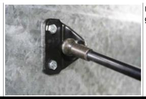
Use 6mm bolts, washers and split rings to fix the gas strut to the trailer wall.
